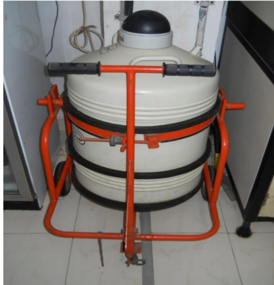
Trolley for LN 2 Dewar movement
