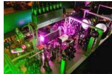
The Texas Petawatt Laser based on Optical Parametric Chirped Pulse Amplification (OPCPA)
