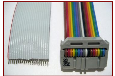
20 way Grey Ribbon cable, rainbow cable with IDC
