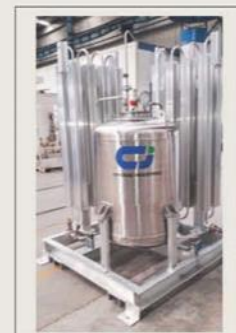
Hexane separation system
