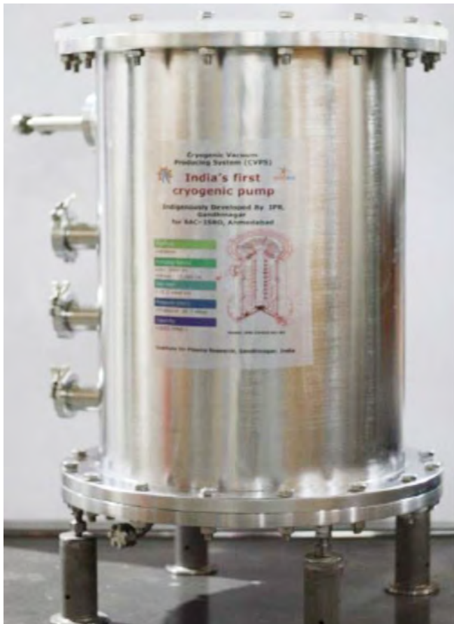
Figure A.1.6 CVPS -400 mm –opening Liquid nitrogen based cryopump
