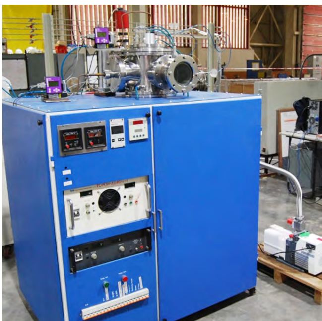
Figure A.4.2.1 High temperature reactive magnetron sputter coating system developed in-house.
