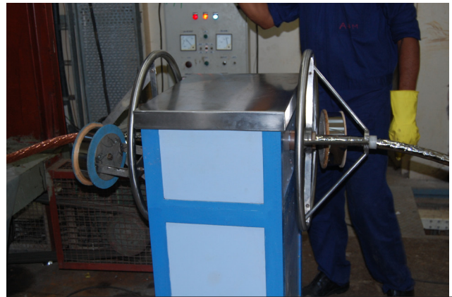
Figure A.2.1.1. 30000 A CICC final stage wrapping.
