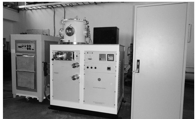
Figure B.1.1.4. Plasma Aluminizing system with unipolar high voltage pulsed power supply for substrate biasing installed in FCIPT.
