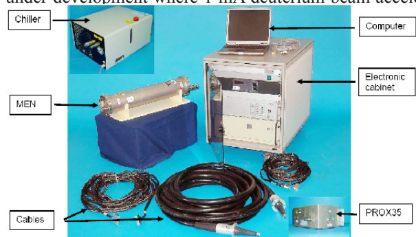
Figure A.2.5.1 The 14 MeV Neutron generator (GENIE35) with subassemblies
