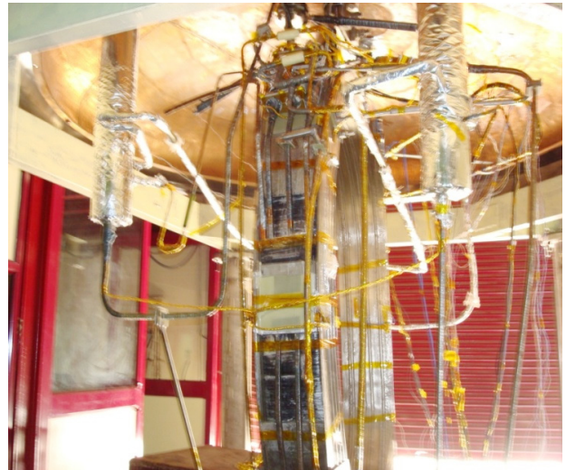
Figure A.1.2.2.1 A fully assembled magnet is getting prepared to be tested
