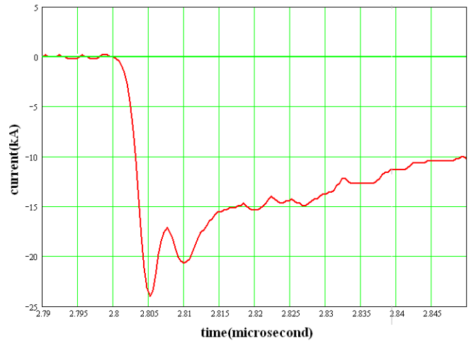
(b) current in the diode, when VIRCATOR is in operation.
