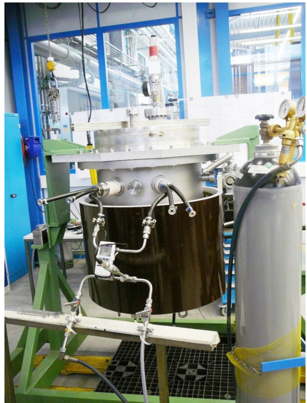
Figure A.2.4.6 Accelerator assembly of ROBIN ion source under pressure testing at the works of M/S Tepla
