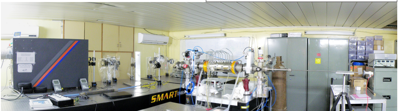
Figure A.3.3.1 View of the plasma accelerator laboratory showing the ArF laser and the plasma chamber.
