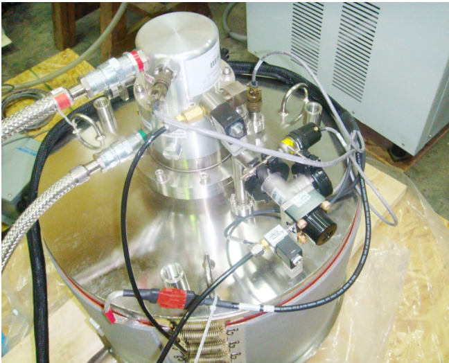
Figure A.2.4.3 Adsorption cryopump for negative ion source experiments
