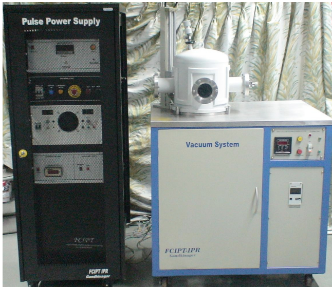
Figure B.1.1.1. Photograph of the Pulsed Plasma Nitriding System that was installed at Delhi University, New Delhi
