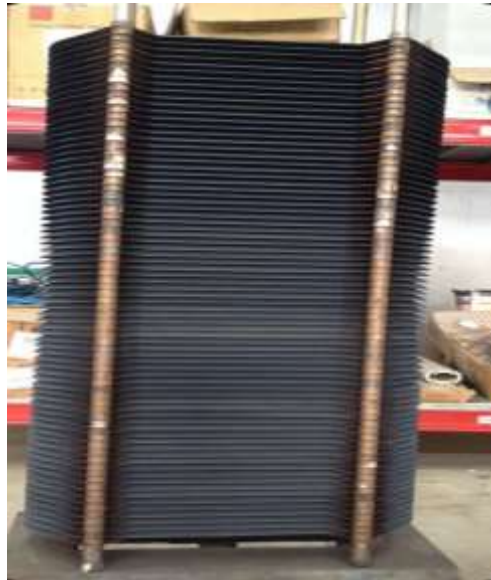
Fig. 9: The photograph of indigenously developed vacuum brazed Cryopump assembly.
