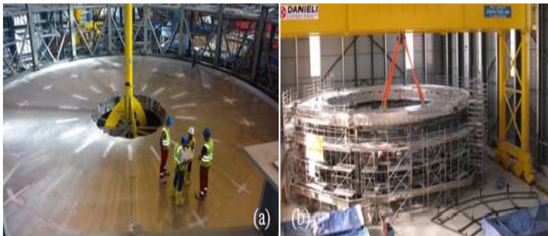
Fig. 27: Base section Tier-1 sandwich structure welding completed at OTER site workshop (a) and Base section Tier-2 setup completed and cleared for welding(b).
