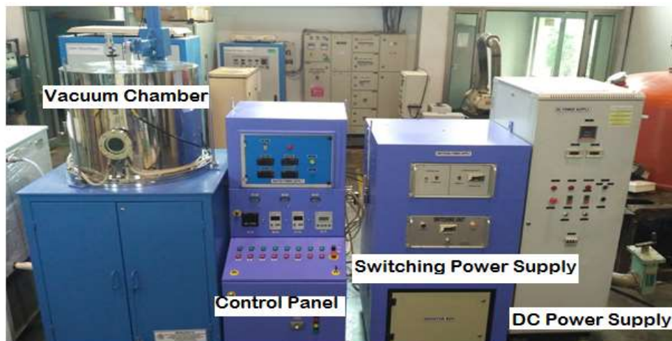
Fig.15: Indigenously developed plasma nitriding system for ISRO Inertial Systems Unit (IISU, Trivandrum).
