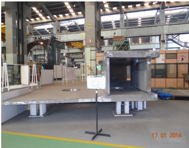
Figure B.2.1 Cryostat Base Section Mockup
