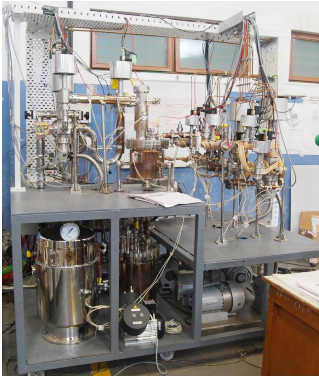
Figure A.2.10.5 Hydrogen isotope permeation experimental set-up
