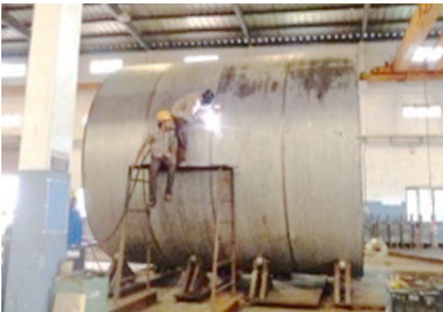
Figure A.2.7.3.1 Manufacturing of the INTF Vacuum vessel at vendor's site.
