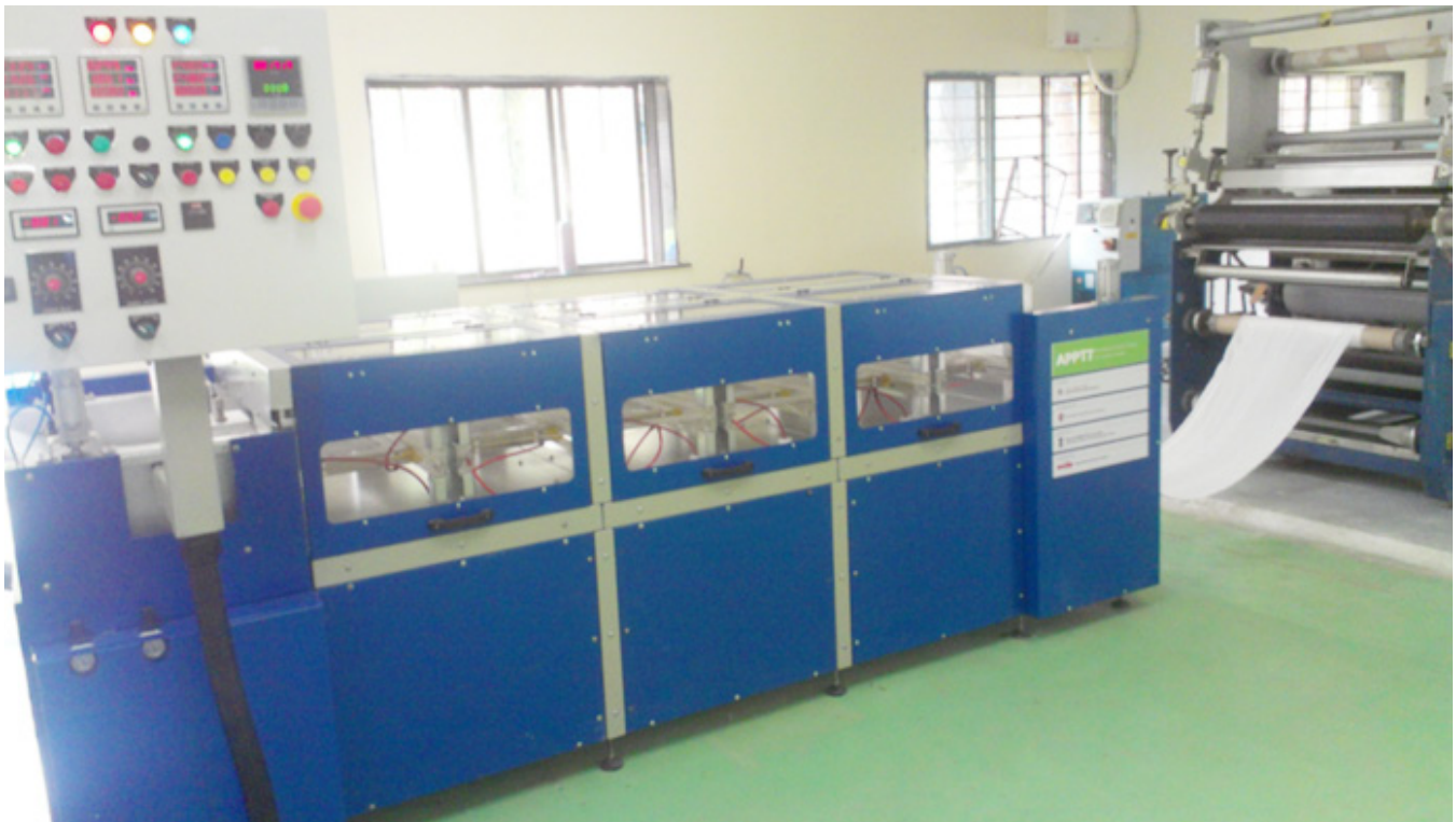
Figure B.1.1 Plasma reactor for textile treatment developed by FCIPT, IPR and functioning at MANTRA, Surat.
