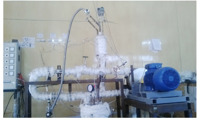
Figure A.2.4.3 Pb-Li loop for testing diagnostics
