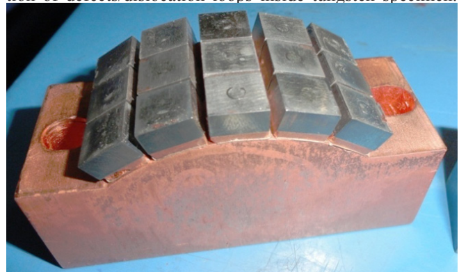
Figure A.2.2.3 Curved Tungsten Macro-Brush brazed with CuCrZr substrate
