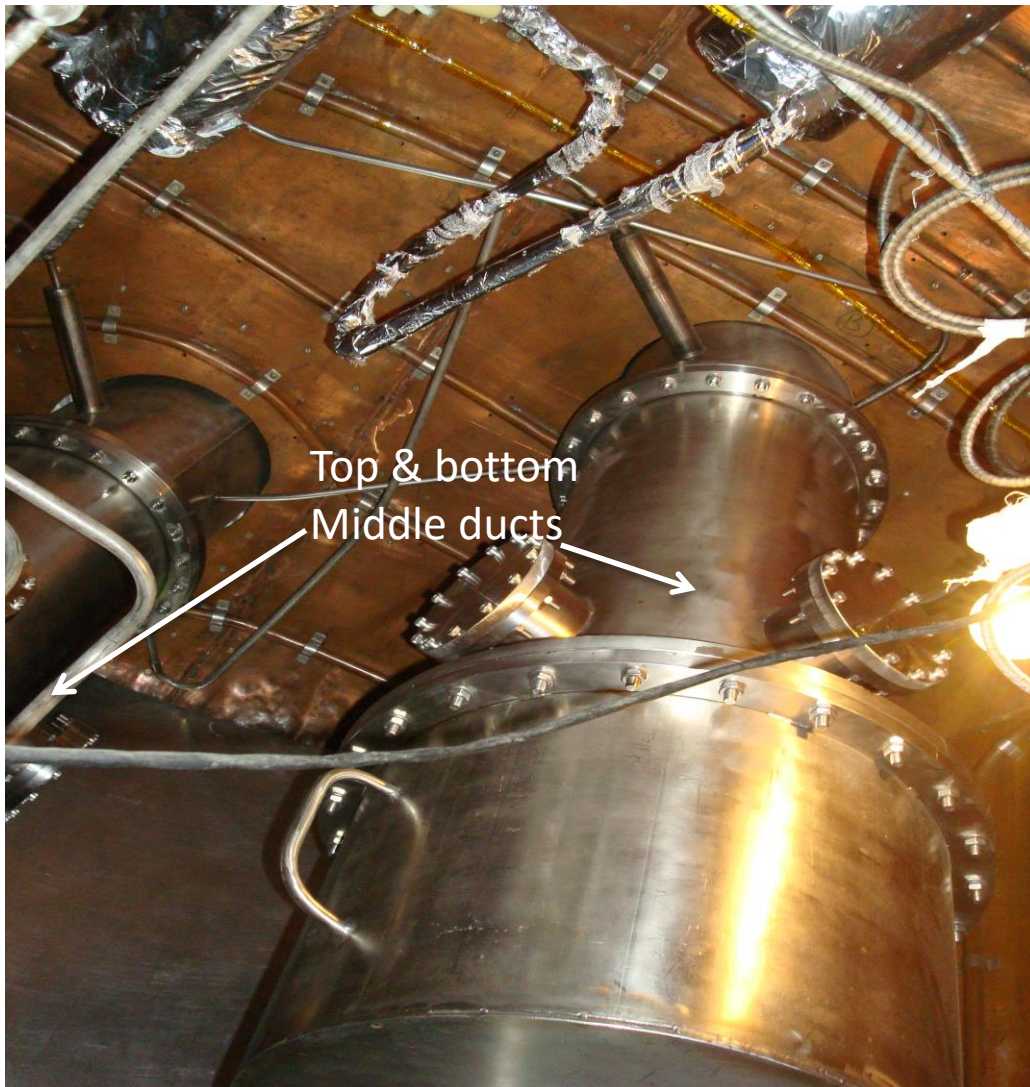
Figure-3 Top and bottom middle ducts inside CFS chamber
