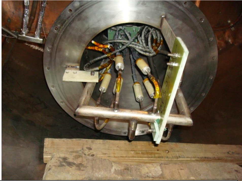
Figure-4 Separation of PF hydraulic paths using G10 supports
