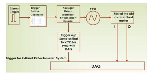
Master Trigger- The complete system should be controlled by an external TTL trigger.
