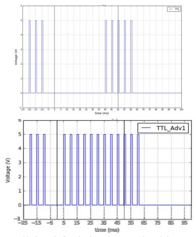
programmable time axis. Sample trigger patterns are shown below.
