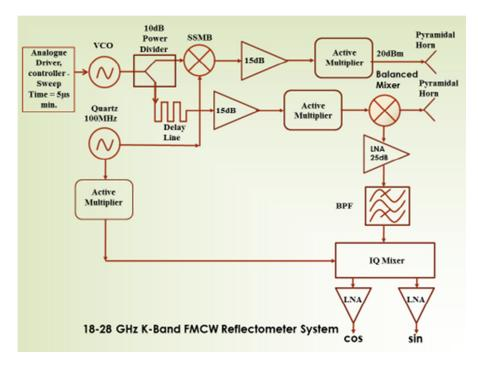
Analog Driver should sweep linearly or accept a txt/csv file containing arbitrary ramp of 1000 points to sweep the VCO. Minimum sweep time must be 5µs. Sample arbitrary ramp pattern as shown below.
