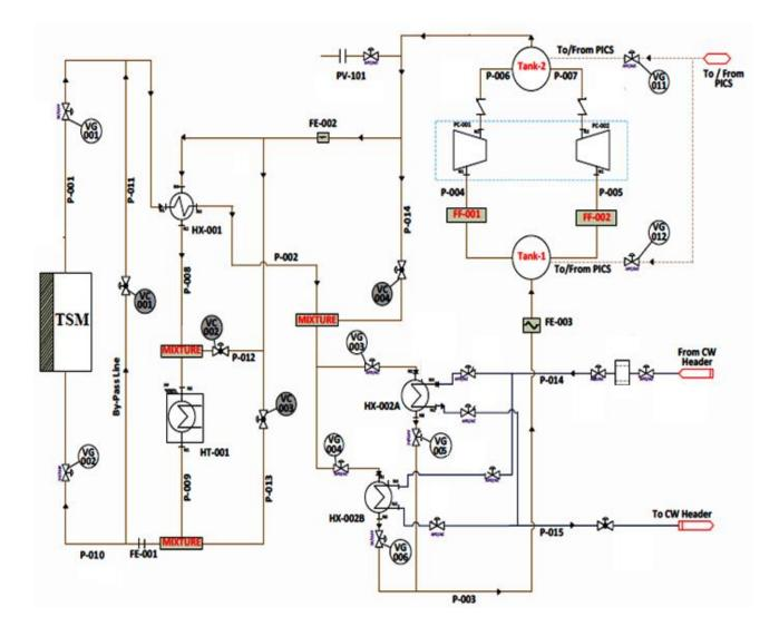
Fig. 1: Flow diagram of main loop of EHCL
