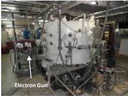
200kW Electron gun horizontally mounted on vacuum chamber of HHFTF
