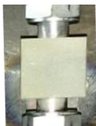
Tungsten coated Stainless Steel test mock-up ( 30 \times 30\text{mm}^2 )
