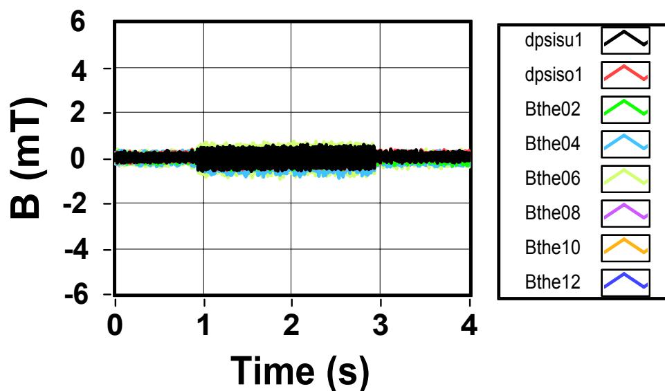
**Difference in calculated and measured probe signal when accounting for low pass filtering of vacuum vessel**
