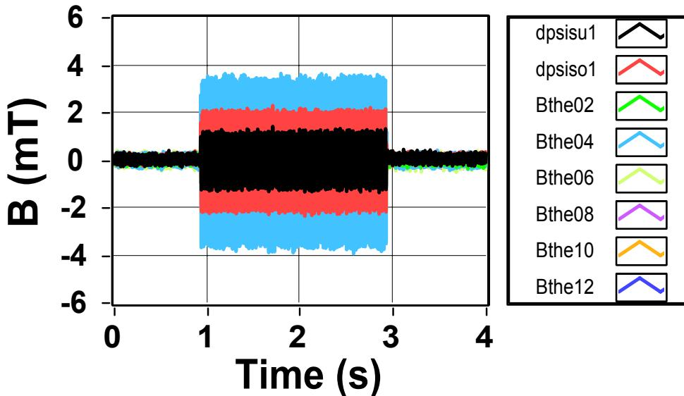
**Difference in calculated and measured probe signal without accounting for low pass filtering of vacuum vessel**
