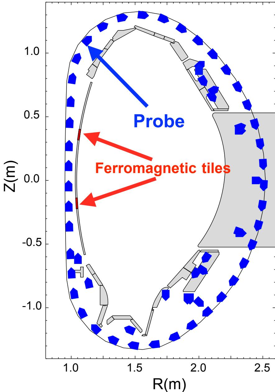
Two rows of low cost, low activation, neutron resistant **ferromagnetic material (P92)** EUROFER foreseen for DEMO
