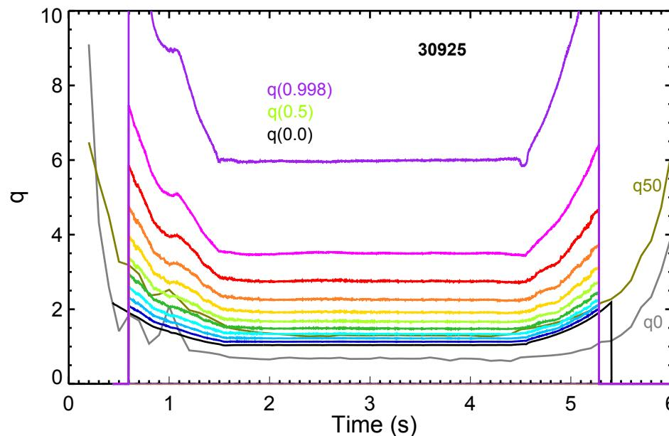
**Comparison of time evolution of offline EQH ( $q_0, q_{50}$ ) and real-time EQR  $q(r)$  profiles show that the offline  $q_0$  can significantly differ from 1**
