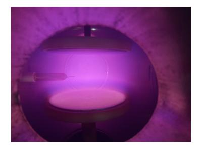
Glow Discharge plasma systems in universities and colleges will provide an opportunity for students to understand the basics of plasma. This will also help them to understand the generation of DC low pressure plasma and its properties using Langmuir probe diagnostics.
