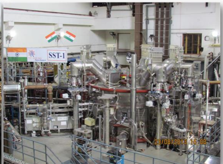
SST-1 equipped with the divertor pumping system
