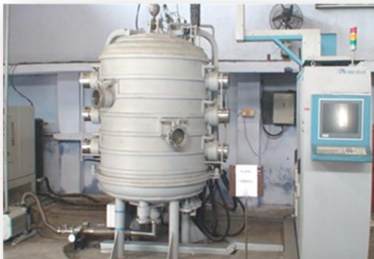
Recently installed Industrial Scale Plasma Nitriding Reactor at the Central Tool Room, Ludhiana
