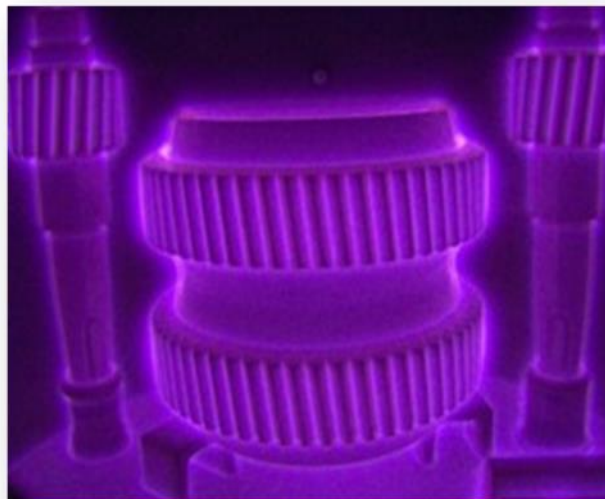
Gear parts undergoing plasma nitriding at FCIPT
