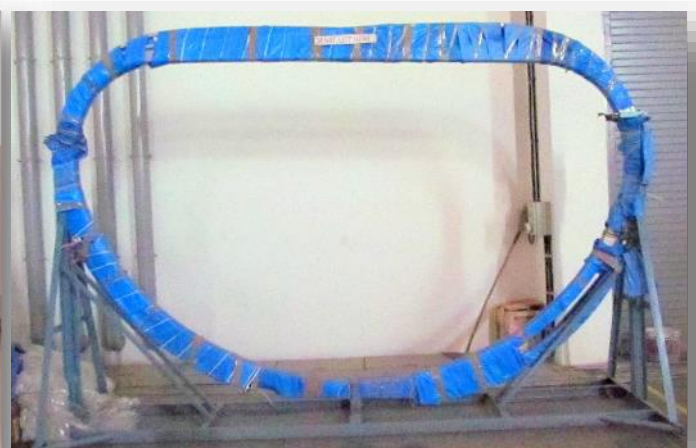
D-shaped NbTi Superconductor CICC for TF Magnet. The dimensions of D-shape magnet are: height \sim 4 m; width \sim 2.5 m
