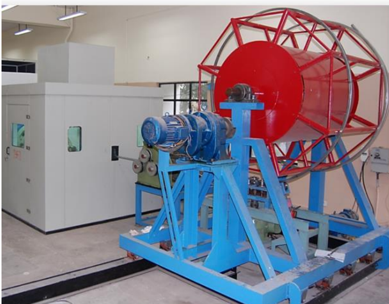
On-line CICC Fabrication Facility developed at AFD, BARC
