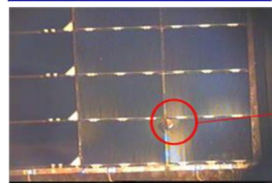
Developed facility, DSO traces during arc, Evolution of the major Arc (SAS = 80 V, Bias = -407 V) at a plasma density of \sim 1 \times 10^6 \text{ cm}^{-3} .
