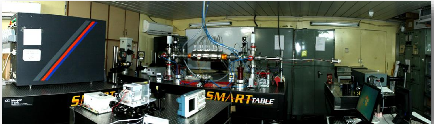
View of the Accelerator laboratory. The excimer laser and the lithium plasma source can be seen in the photograph.
