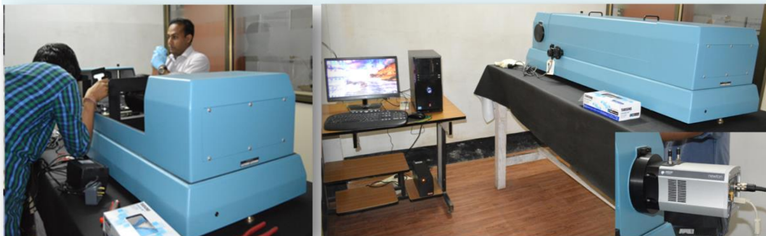
The complete spectrometer setup after installation; Inset (right side bottom) shows the CCD.
