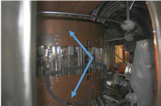
**Top & Bottom Inner divertor plate installed in SST-1 Vacuum Vessel**
