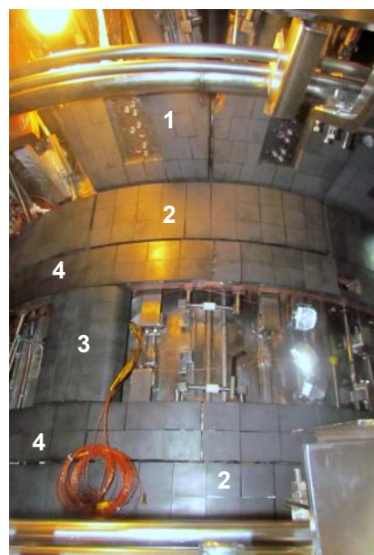
Installed components: (1) Main baffle (2) IDP- Inboard divertor plate (3) Inboard Limiter (4) IPS- Inner passive stabilizer
