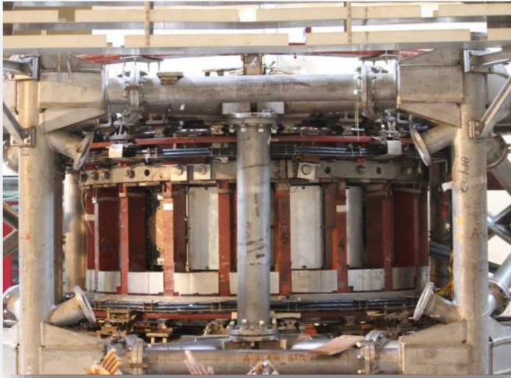
The support structure, coils and the vessel of Aditya now visible after the diagnostics have been removed.
