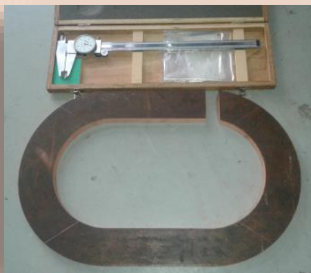
40 mm thick SS316LN plate machining and 19mm thick ETP copper (pulse power)
