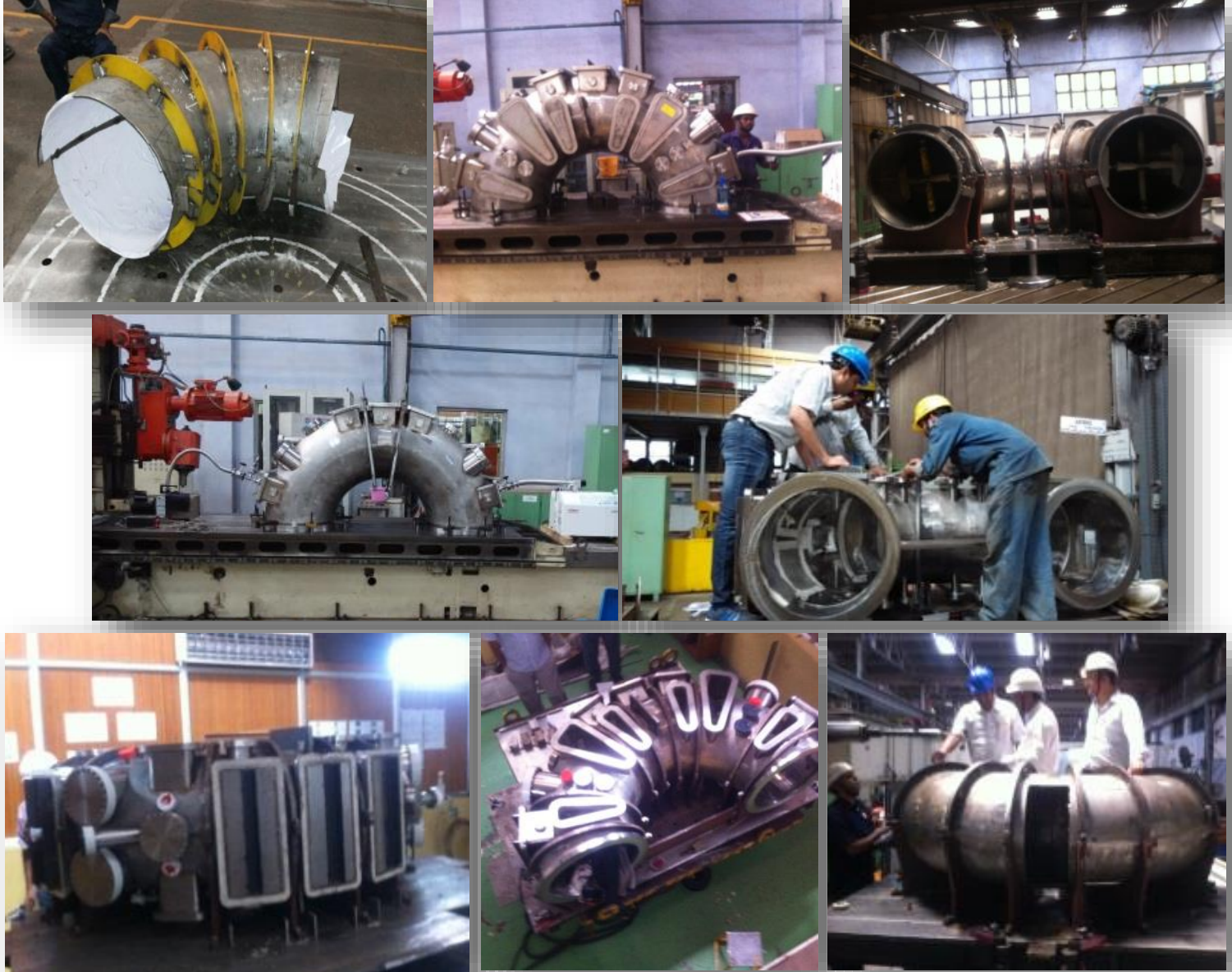
Images of the new vacuum vessel for Aditya under fabrication and testing at M/s Godrej & Boyce Ltd., Mumbai.
