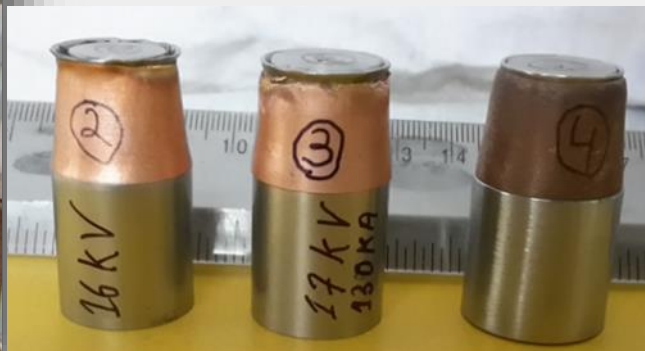
(L) The EM pulse welding setup. (R) The samples of welded SS D-9 samples using this setup.
