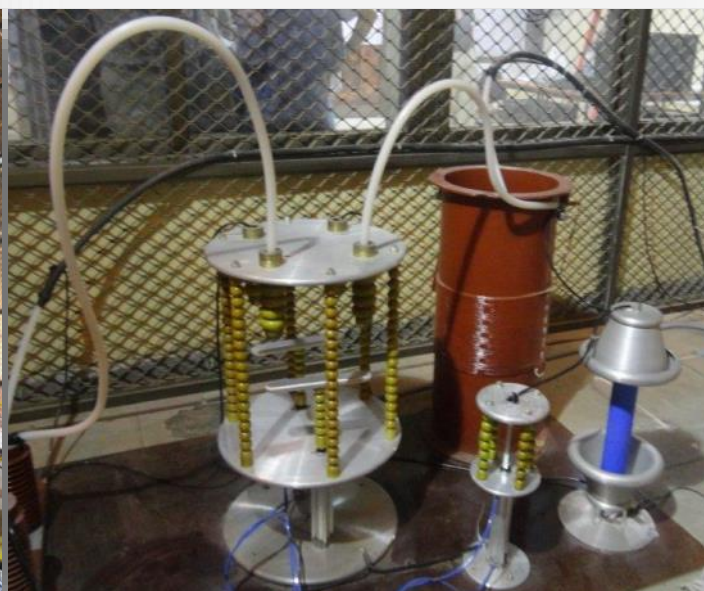
(L) The HV power supply during installation at BARC. (R) The HV isolator and ground switches of the system
