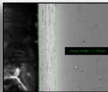
(L) SEM image (cross-section) showing the thickness (2.1 μm) of the film. (R) SEM image (top surface) showing uni-
