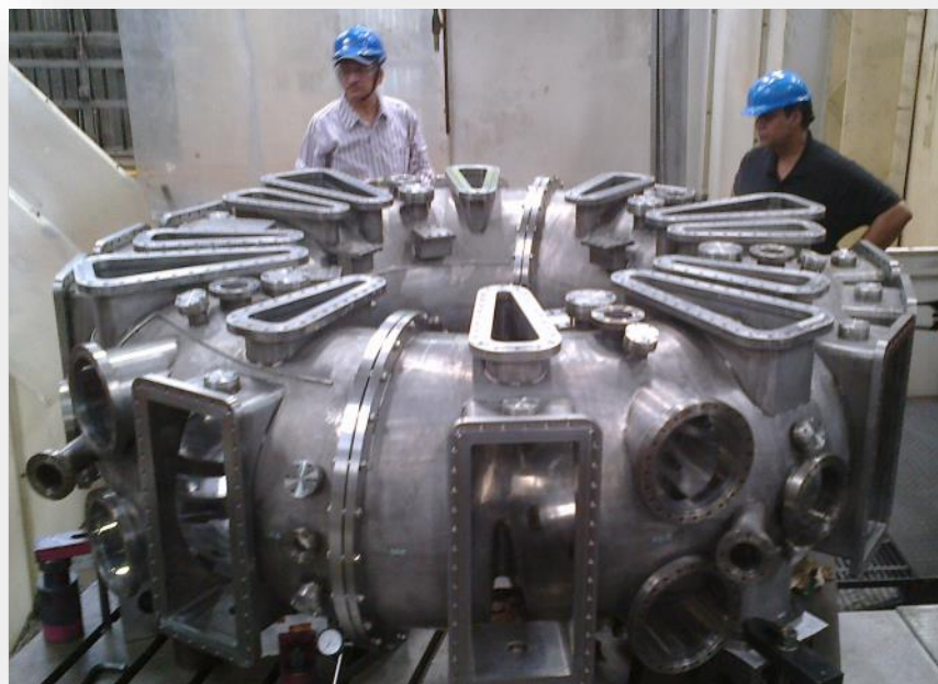
(L) Torus Assembly of vacuum vessel for Aditya Tokamak as on 20-7-2015 (R) The old Aditya vacuum vessel after dismantling.
