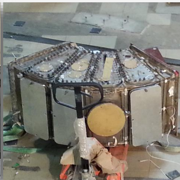
(L) Torus Assembly of vacuum vessel for Aditya Tokamak as on 20-7-2015 (R) The old Aditya vacuum vessel after dismantling.
