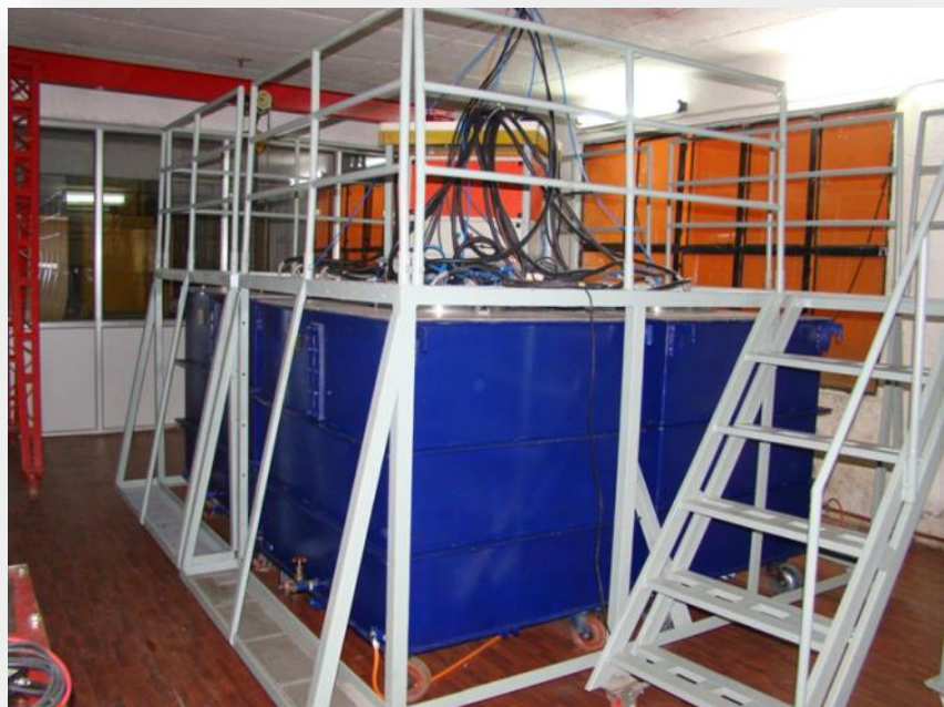
(L) The EM pulse welding setup. (R) The samples of welded SS D-9 samples using this setup.
