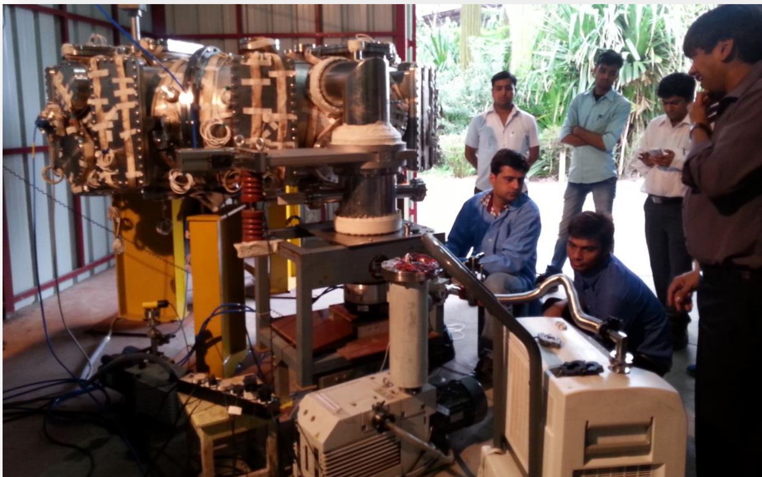
The new vacuum vessel of Aditya undergoing vacuum tests at IPR.
