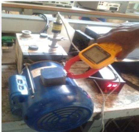
Current, Temperature and Vacuum measurements using the converted Indian motor
