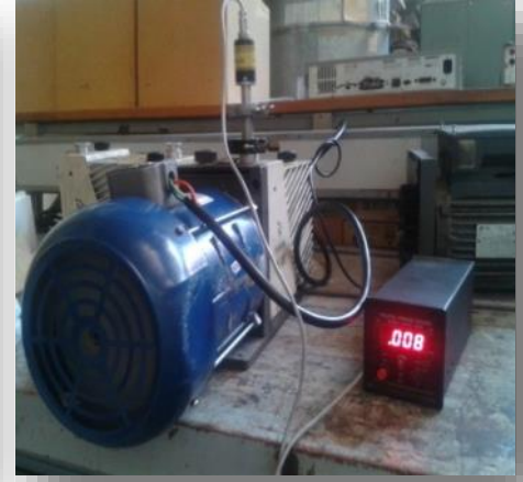
Current, Temperature and Vacuum measurements using the converted Indian motor
