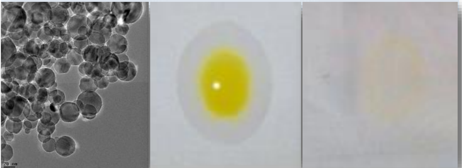
Picture shows the electron microscopy image of titania nanoparticles (left side) followed by turmeric stain on nanotitania coated fabric before (middle) and after exposure to sunlight (right side)
