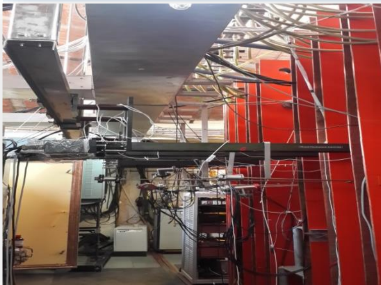
(L) Integrated probe positioning system installed on the LVPD. System. (R) Stepper Motors for controlling translators motion.
