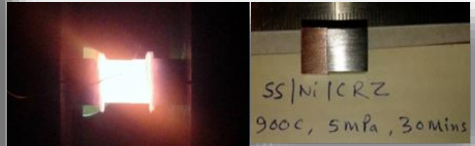
(L) Diffusion bonding experiment at Gleeble machine (R) Diffusion bonded specimen
