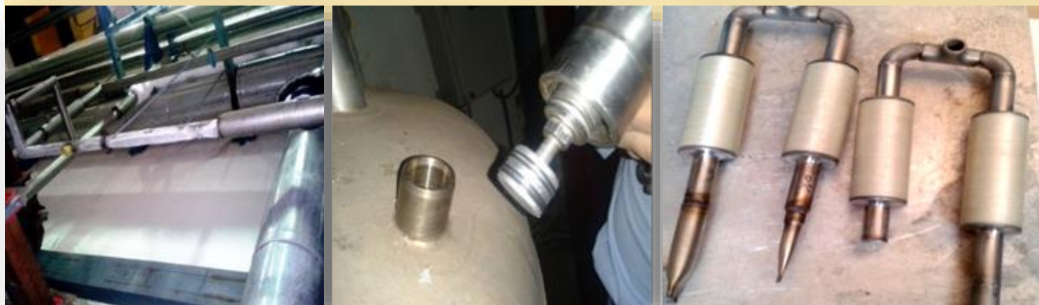
(L-R) Frosted cryogenic lines, Puppet valve assembly and In-house developed isolators
