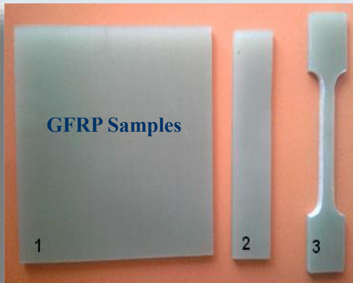
(Above) GFRP insulation material samples for testing (1) Breakdown strength (2) Shear strength (3) Tensile strength.
