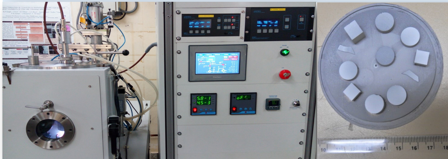
(L) Magnetron sputtering Unit (R) Ti sputtered samples
