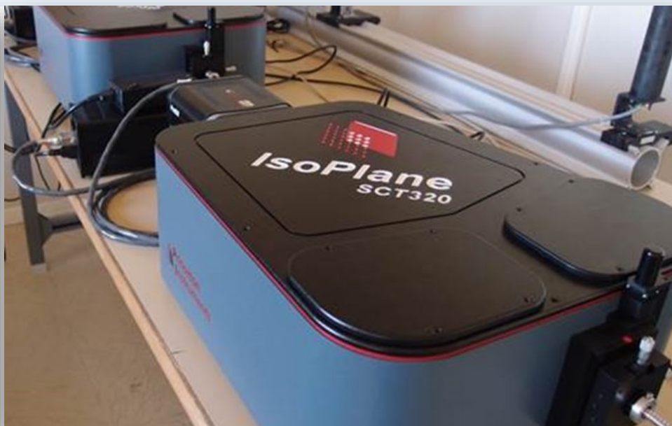
Left : The optical fiber array for viewing the plasma facing components. Right : The visible spectrometer assembly
