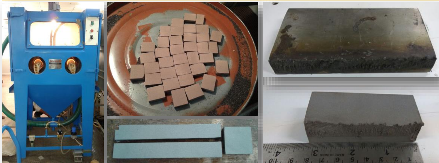
(L-R) : The sandblasting machine ; Copper (top) and tungsten (bottom) samples after sandblasting ; Plasma cut SS block before (top) and after (bottom) sand blasting.
