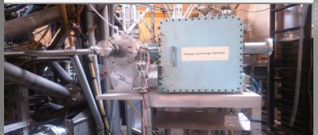
(Clockwise) The layout of CXD-NPA system for SST-1 ; Temporal evolution of core-ion temperature T_{i0} and T_{e0} for Plasma Shot#29387 of Aditya Tokamak; Image of the CX-NPA diagnostics on Aditya Tokamak.
