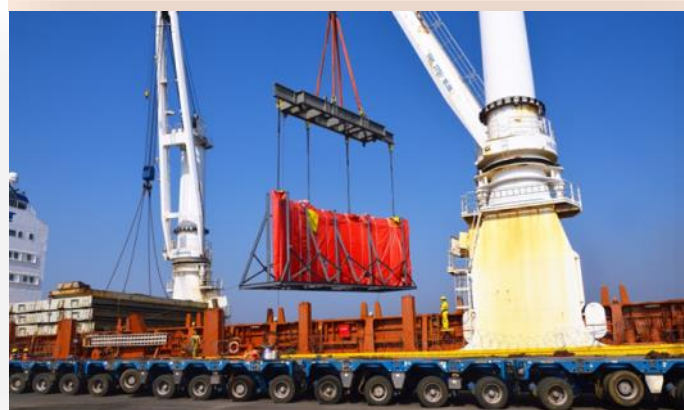
(L) Loading of one of the six Cryostat Lower Cylinder Tier-1 sectors at Hazira port (R) Unloading of the sectors in the Cryostat Workshop at ITER site
