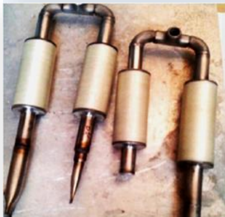
(L-R) Developed Electrical Insulation breaks ; Breaks Installed in upgraded PF coils hydraulics ; Thermal shock testing at 4.2 K in the Lab
