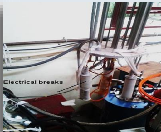
(L-R) Developed Electrical Insulation breaks ; Breaks Installed in upgraded PF coils hydraulics ; Thermal shock testing at 4.2 K in the Lab
