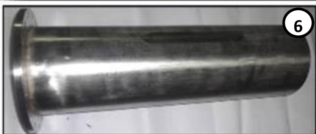
Fabricated components of the axial valve : (1) Schematic of the axial valve (2) Bellow mounting adapter (3) Seal mounting flange (4) Bellows (5) Pneumatic actuator assembly (6) Bellow guiding cylinder (7) Guide for bellow (8) Valve (9) Bush
