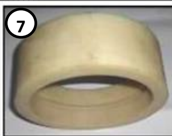
Fabricated components of the axial valve : (1) Schematic of the axial valve (2) Bellow mounting adapter (3) Seal mounting flange (4) Bellows (5) Pneumatic actuator assembly (6) Bellow guiding cylinder (7) Guide for bellow (8) Valve (9) Bush
