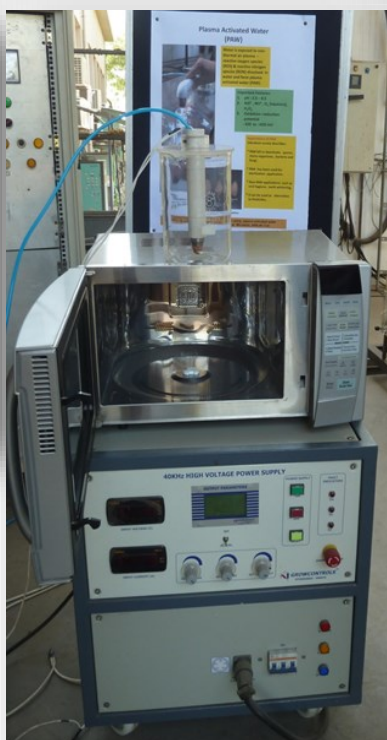
The device developed at FCIPT to generate PAW
