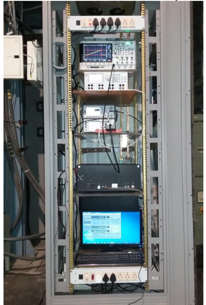
Images of the rack mounted microwave electronics as well as the data acquisition system for the reflectometry setup.
