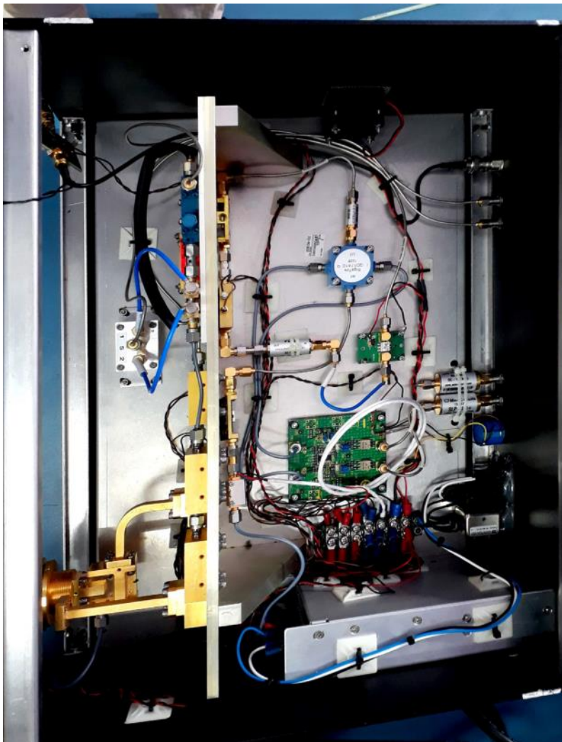
Images of the rack mounted microwave electronics as well as the data acquisition system for the reflectometry setup.
