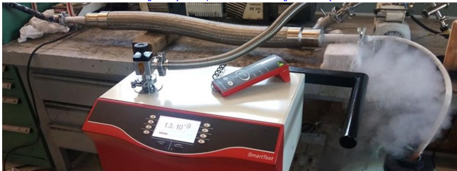
Vacuum and He leak tightness performance being carried out at 77 K
