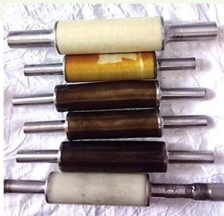
(L) Fabrication of IB (M) In-house developed IB's (R) Helium leak tightness performance test at 77 K, 10 bar (g) pressure
