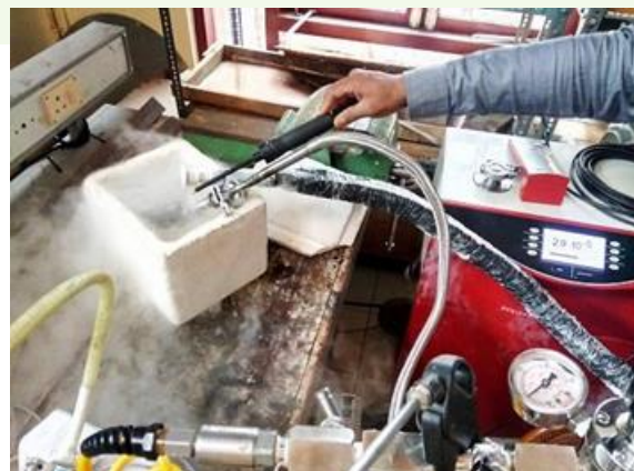
(L) Fabrication of IB (M) In-house developed IB's (R) Helium leak tightness performance test at 77 K, 10 bar (g) pressure
