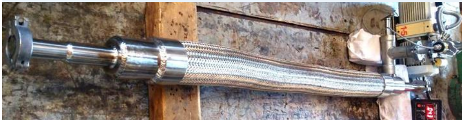
Indigenously developed 1" NB / 1.2 m long Flexible Cryo Line
