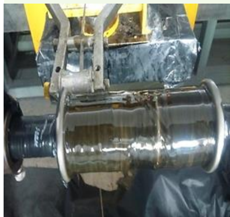
(L) Fabrication of IB (M) In-house developed IB's (R) Helium leak tightness performance test at 77 K, 10 bar (g) pressure
