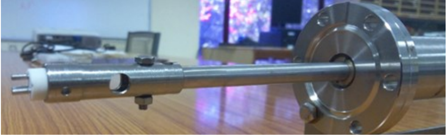
Assembled actuator with the Langmuir probes
