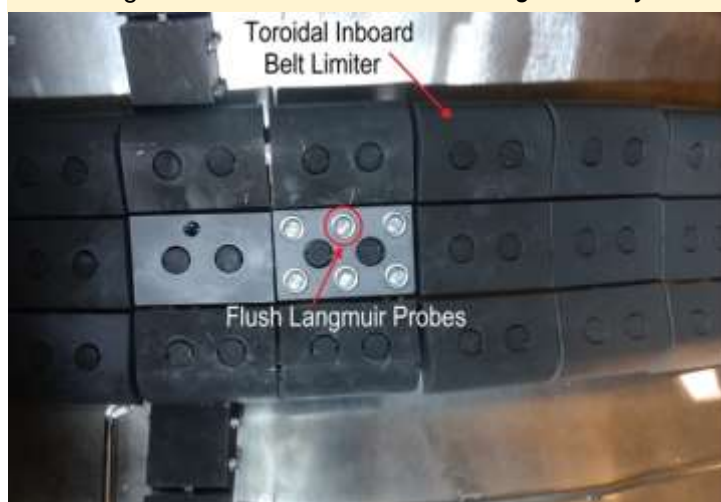
(L) The toroidal inboard belt limiter installed inside the Aditya-U tokamak showing the installed six flush mounted Langmuir probes on a graphite tile (R) Thermal image of the same toroidal inboard belt limiter during the plasma disruption in a typical Aditya-U discharge # 31201.
