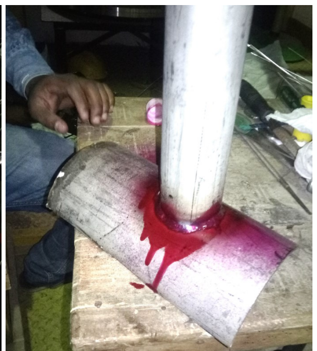
(L) Welding of 80 K Return Lines to LN2 Phase Separator (R) Dye penetration NDT test of the line
