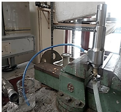
Vacuum Performance test of Rupture Disc, Pressure Safety Valve and ORS Filter System of Helium Compressor Unit SST-1
