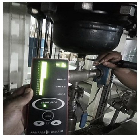
Vacuum Performance test of Rupture Disc, Pressure Safety Valve and ORS Filter System of Helium Compressor Unit SST-1
