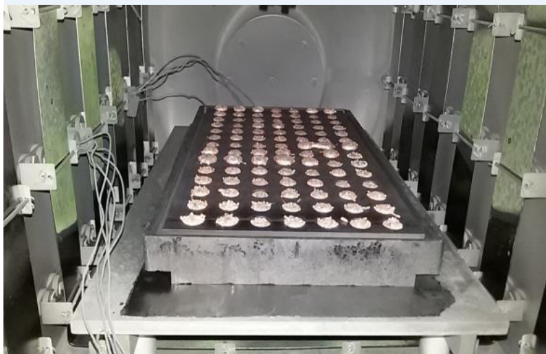
(Top) The completed Cu-W electrode (L) The batch casting of the electrodes in progress (R) Copper cast on tungsten rod
