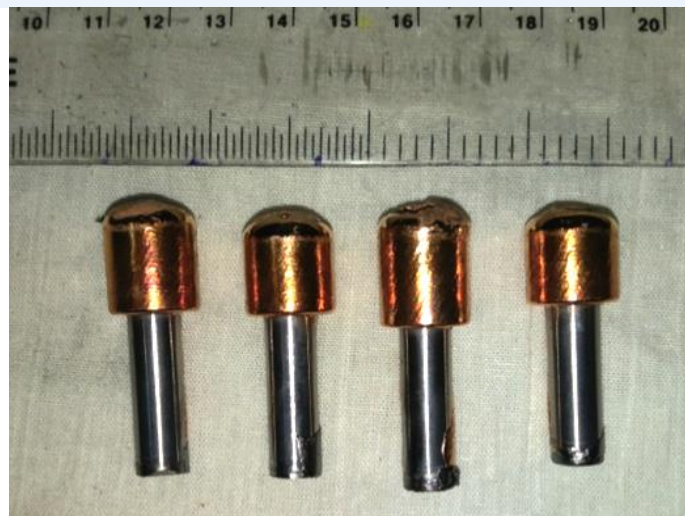
(Top) The completed Cu-W electrode (L) The batch casting of the electrodes in progress (R) Copper cast on tungsten rod
