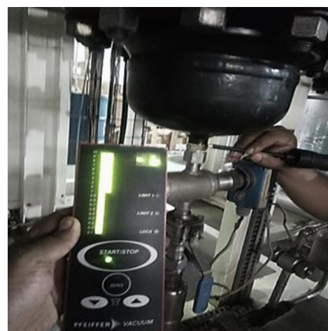
Vacuum Performance test of Rupture Disc, Pressure Safety Valve and ORS Filter System of Helium Compressor Unit SST-1
