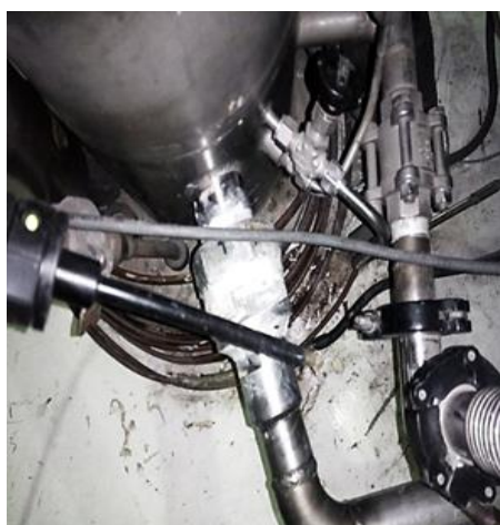
Vacuum Performance test of Rupture Disc, Pressure Safety Valve and ORS Filter System of Helium Compressor Unit SST-1
