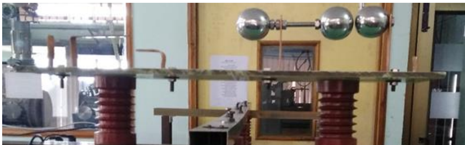
Arrangement for wire burn and arc test
