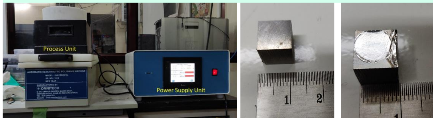
(L) The Electro Polishing and Etching Machine (R) SS316L sample before and after electro polishing
