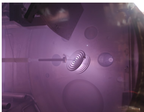
The antenna assembly being tested at (L) 60 MHz, 850W (M) 260 MHz, 100W and (R) 403 MHz, 100W
