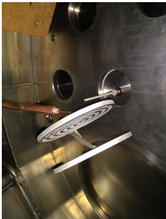
(L) Prototype spiral antenna installed at the 1/8th of SST-1 section (R) Langmuir probe data using this antenna system
