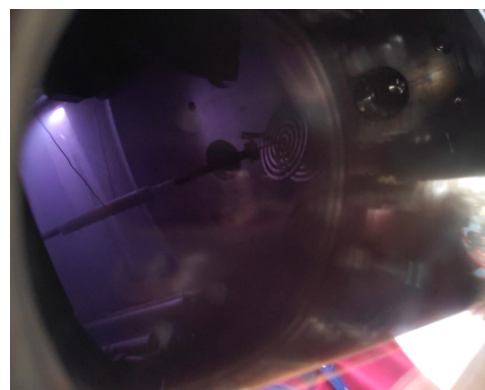
The antenna assembly being tested at (L) 60 MHz, 850W (M) 260 MHz, 100W and (R) 403 MHz, 100W
