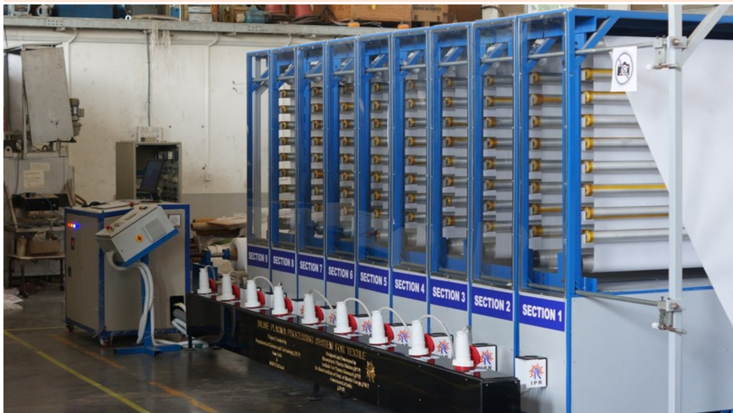
Plasma system developed by IPR for inline treatment of textiles
