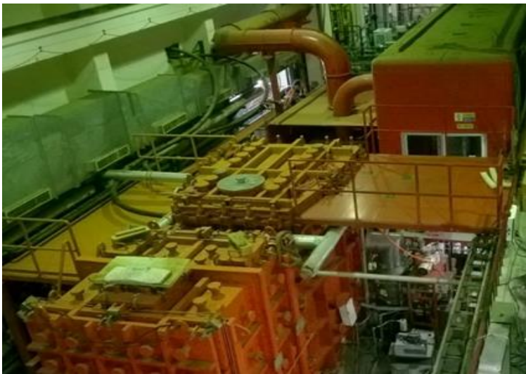
(L) The SST-1 NBI test stand (R) Image of the 38 kV beam
