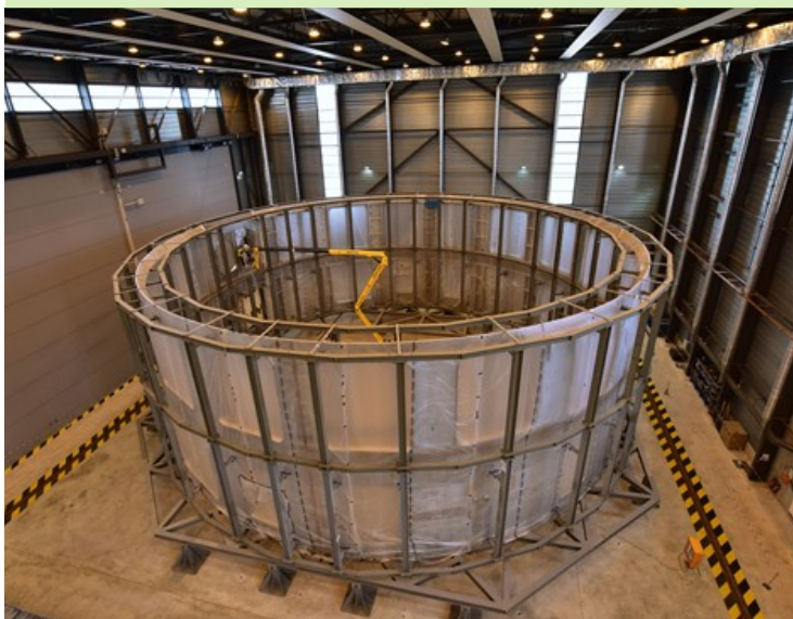
(L) Cryostat Lower Cylinder-subassembly completed at Cryostat workshop, ITER site, France (R ) 12 such sectors of Upper Cylinder dispatched from India
