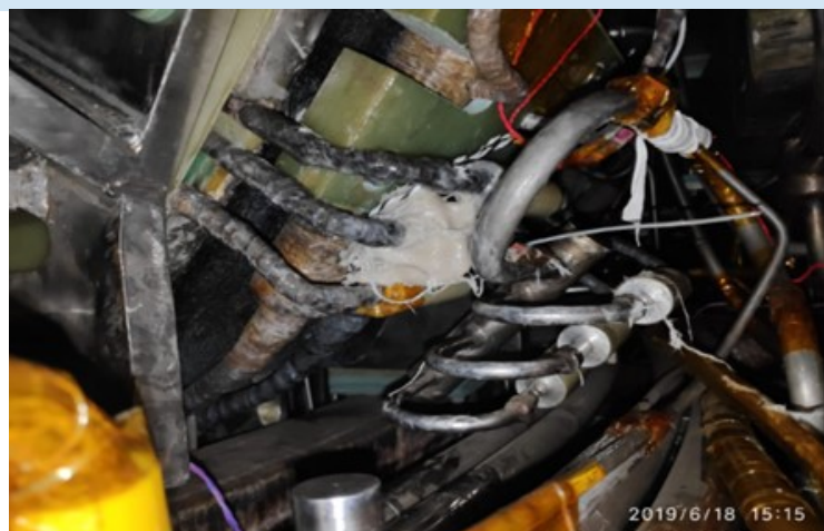
(L) Location of Helium leak at Electrical Break interface (R) Repaired Electrical Break interface
